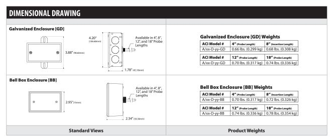
Note: There are two enclosures included with configurations involving Temperature Transmitters. A secondary GD (Galvanized) enclosure contains the transmitter board to protect it from the extreme temperatures exposed to the sensing element
