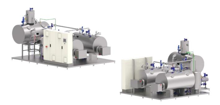
Dpstar electric heater steam boilers are used in industry when the primary available energy is electricity. The steam is generated by an electric resistor heating flange inside the boiler shell. The units are skid-mounted complete with feed water tank, water treatment and control panel. The complete factory pre piping and wiring ensures quick and easy installation on site.
