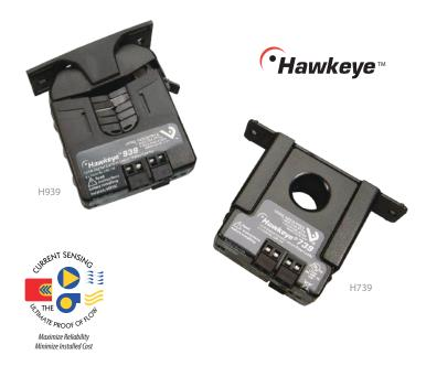
Hawkeye Relay Combination Series high voltage output current switches are the ideal solution for the automation installer. These units combine a current switch and relay into a single package, reducing the space required for total control of fans and pumps. The integrated current switch and relay operate independently of one another. All relay connections are externally available for maximum flexibility.
