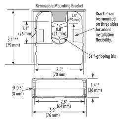
\* Terminal block may extend up to 1/8" over the height dimensions shown.
