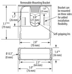
\* Terminal block may extend up to 1/8" over the height dimensions shown.
