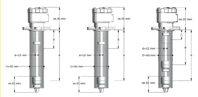
The dimensions A, B and C depend on the ordered version. For one signalling point: A min. 50mm, A max. 1000mm. For two signalling points: A min. 150mm, A max 1000mm; B min. 50mm, B max 900mm; (A – B) min. 100mm. For three signalling points: A min. 250mm, A max 1000mm; B min. 150mm, B max 900mm; C min. 50mm, C max 800mm; (A – B) min. 100mm, (B – C) min. 100mm.
