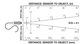
D:S is the optical resolution expressed as a ratio of the distance to the resolution spot divided by the diameter of the spot.
